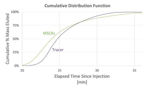
Figure 3: Cumulative effluent mass for tracer and MSCK tests in sand column
